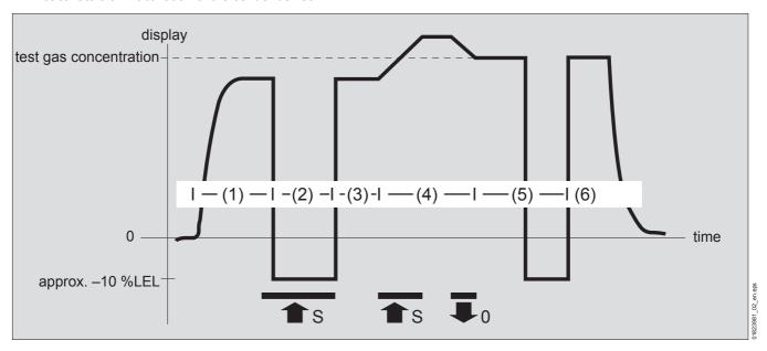
The values in %LEL mentioned in this section are only valid for gas warning systems that are calibrated for the measured gases methane, propane or ethylene. The actual LEL values [%] may deviate from the mentioned LEL values [%] on gas warning systems which have not yet been calibrated or which were calibrated with a substitute gas and a calibration factor.
